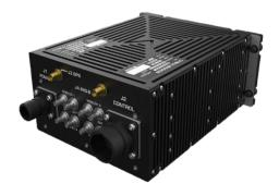
Compact recorder, with low weight of 2Kg (4.4lbs) it allows you to record a lot of parameters in a reduced volume. This unit is capable to record in same time Analog/Digital bus, Video/Audio data.
