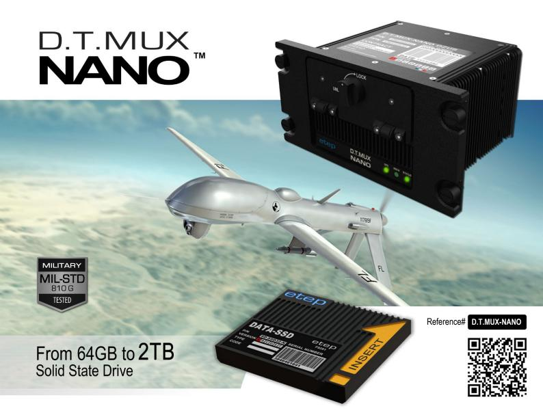
The D.T.MUX Nano Airborne Data Recorder, is a powerful miniature unit (Available in two form factor) with recoding capacity on Solid State Disk (SSD) from 64GB to 2TB, support Military Grade Encryption/Erasure and Physical Destruction. IRIG 106 Chapter 10 Compliant.
